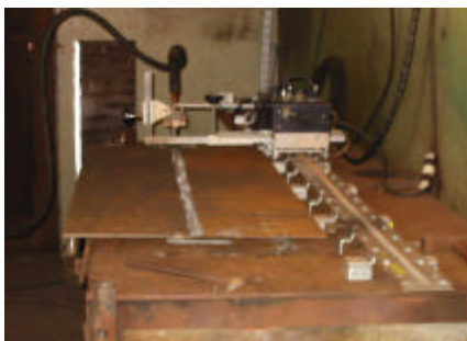
Photos 5 and 6 – The use of run-on and run-off plates.
