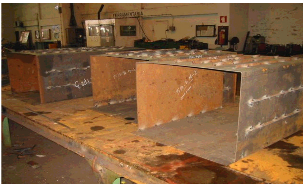
Photographic showing the three box girder models
