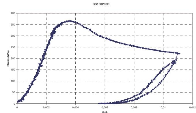
Figure 14 – Final loading and collapse of panel BS150200B.
