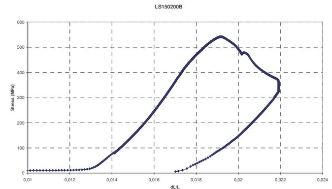
Figure 16 - Stress shortening curve of the LS150200B specimen test. Final cycle of loading.
