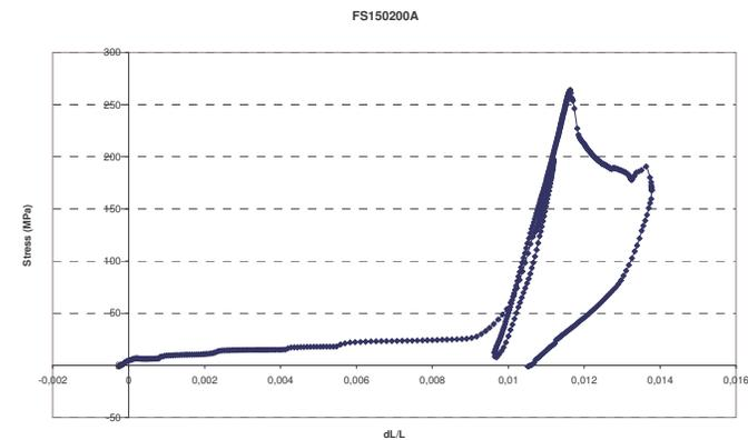
Figure 5– Stress shortening curve of the FS150200A specimen test. All cycles of loading
