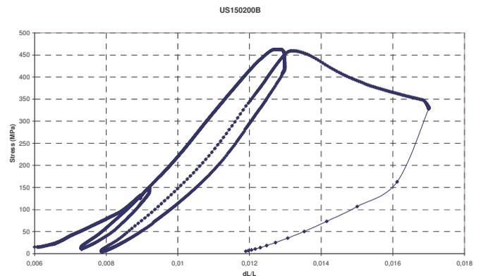
Figure 21 - Stress shortening curve of the US150200B specimen test. All cycles of loading.
