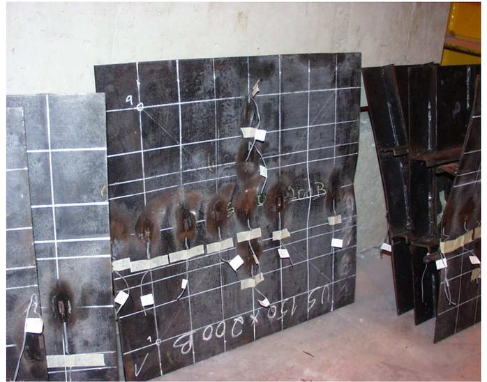
Figure 20 – Final collapse shape of US150200B panel on the plating.
