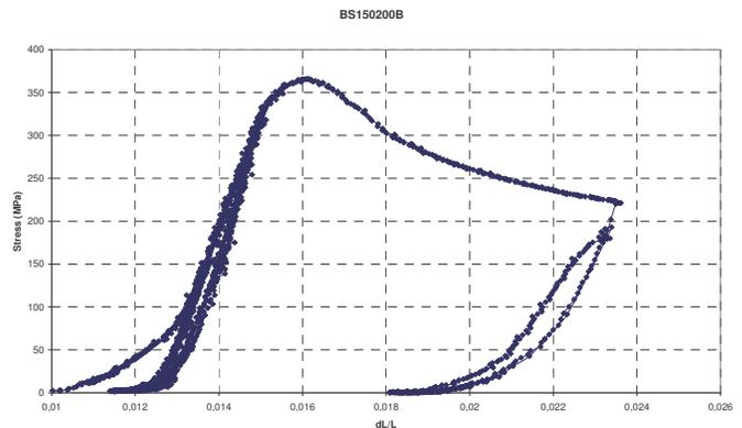
Figure 11 - Stress shortening curve of the BS150200B specimen test. All cycles of loading.
