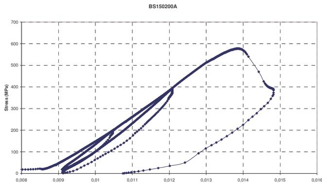
Figure 9 - Stress shortening curve of the BS150200A specimen test. All cycles of loading.
