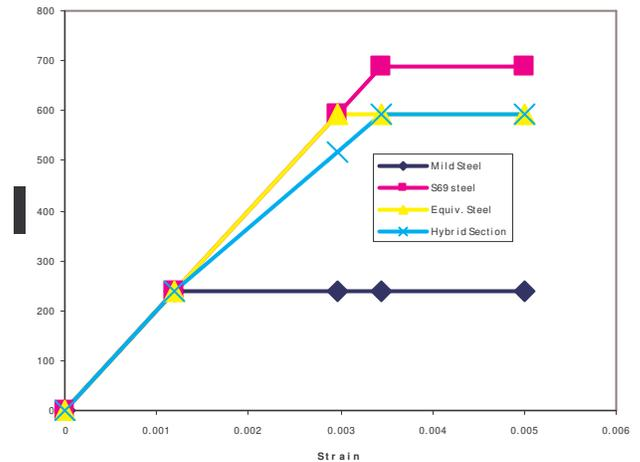
Figure 10 – Material behaviour of mild, S69 steel and comparison with equivalent material of hybrid BS specimens.
