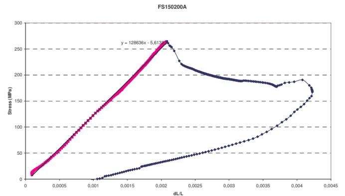
Figure 7 – Final loading and collapse of panel FS150200A
