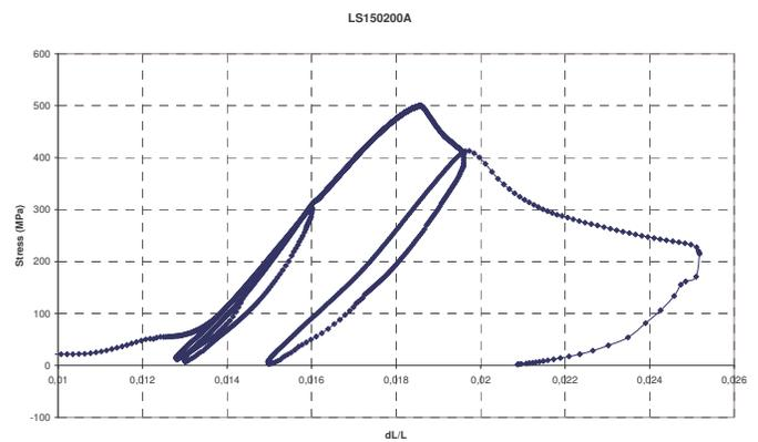
Figure 15 - Stress shortening curve of the LS150200A specimen test. All cycles of loading.
