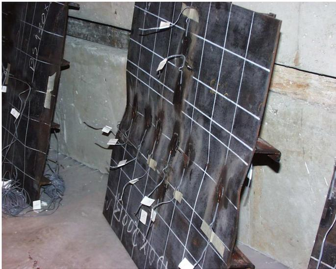
Figure 18 – Collapse shape of LS150200B panel.
