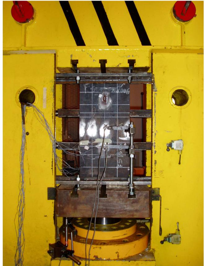
Figure 3 – Setup of the 200 series test of stiffened plates
