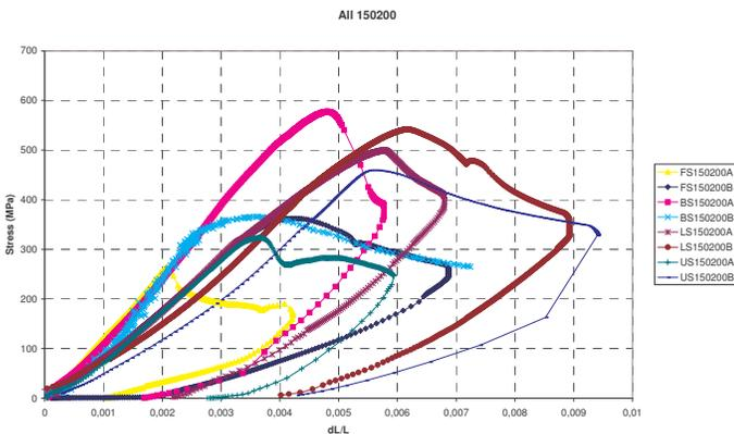
Figure 23 – Average stress strain curves for all 200 series
