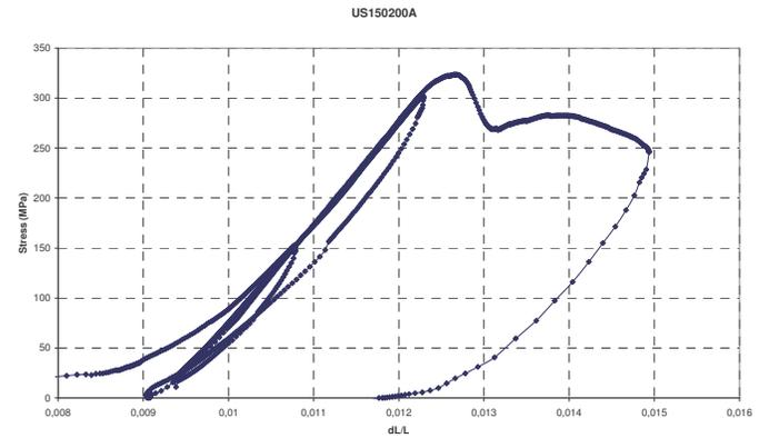
Figure 19 - Stress shortening curve of the US150200A specimen test. All cycles of loading.
