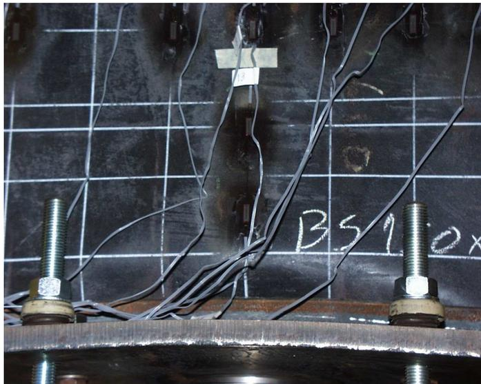
Figure 12 – Premature failure of the loading support leading to premature collapse on the adjacent span of the panel.
