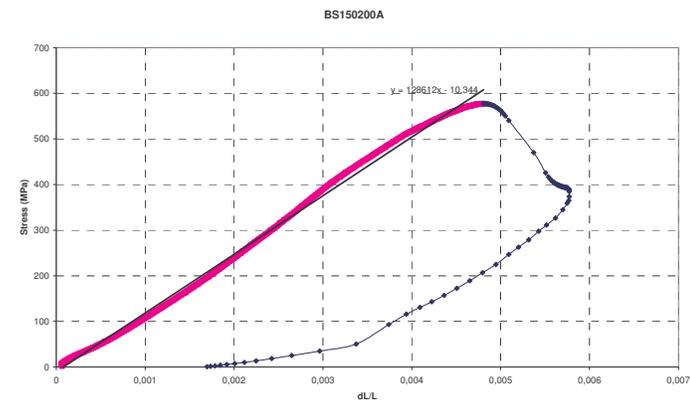
Figure 13 – Final loading and collapse of panel BS150200A.
