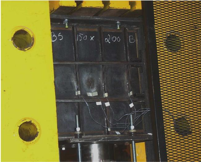
Figure 4 – Details of the lateral support of the frames in vertical guides.
