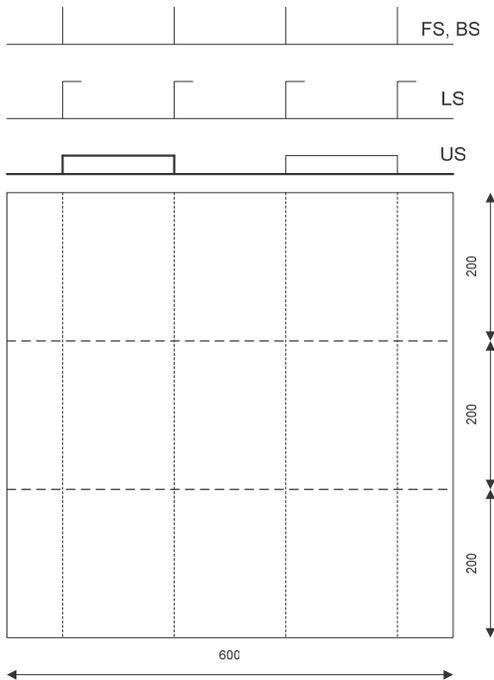
Figure 2 - Geometry of wide stiffened panels.
