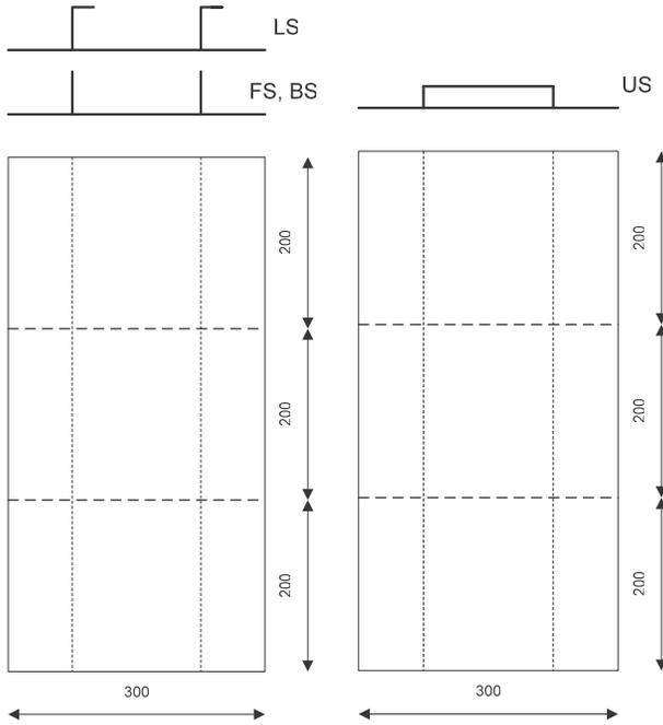
Figure 1- Geometry of narrow stiffened panels for fully S690 steel (FS), mild bar stiffeners (BS), 'L' and 'U' mild steel stiffeners.
