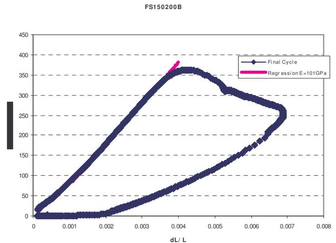
Figure 8 – Final loading and collapse of panel FS150200B
