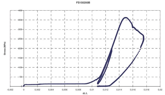
Figure 6 – Stress shortening curve of the FS150200B specimen test. All cycles of loading
